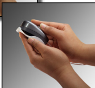
Mounting the ambient light head on a basICColor SQUID2
