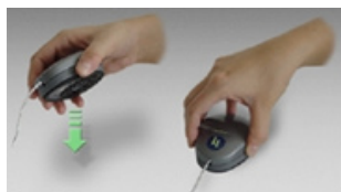
Calibration position for the basICColor SQUID2 (without the translucent base!!)
