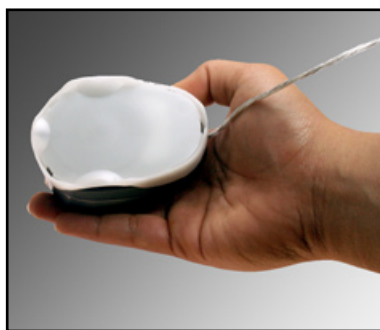
Positioning basICColor SQUID2 for ambient light measurement.
